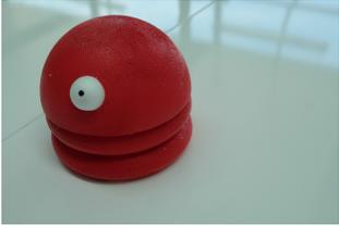
**Figure 4:** A picture of the tangible prototype: a physical device, bearing similarity in appearance with the robot equipped with sensors (speed, rotation, tilt angle), allows the child to control the robot. Direct mapping between the small controller and the big robot results in navigation on the z-plane with rotation and forward/backward movement.
