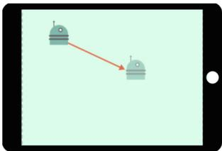
**Figure 3:** A Picture of the GUI: robot locomotion is controlled by drag and drop of the robot icon.
